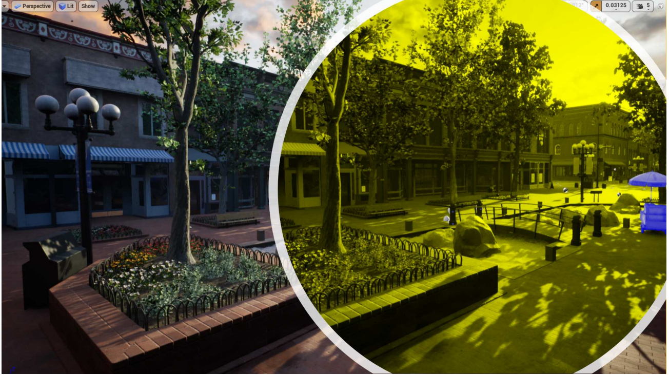
Figure 5: Illustration of RGB image and (yellow image in the circle) false color (red = grayscale, green = grayscale, blue = object ID) stencil buffer for per pixel ground truth.
