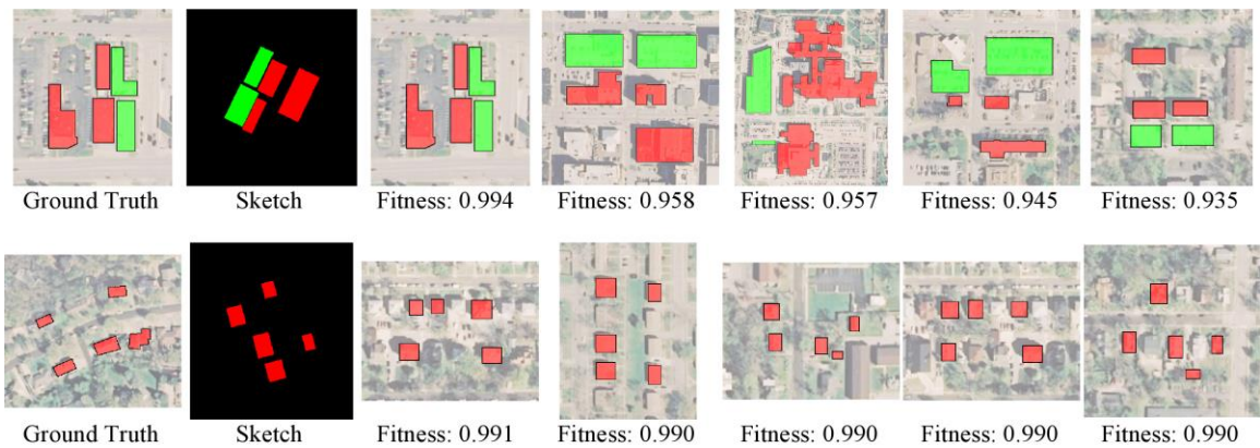
Figure 4.7 Examples of top matches for the simplified sketches. Buildings are shown in red and parking lots are shown in green. The top match is the correct mapping to the ground truth set in the first example, whereas the ideal match is not one of the top scoring matches for the second example. All of the top matches for each example share a similar spatial configuration.
