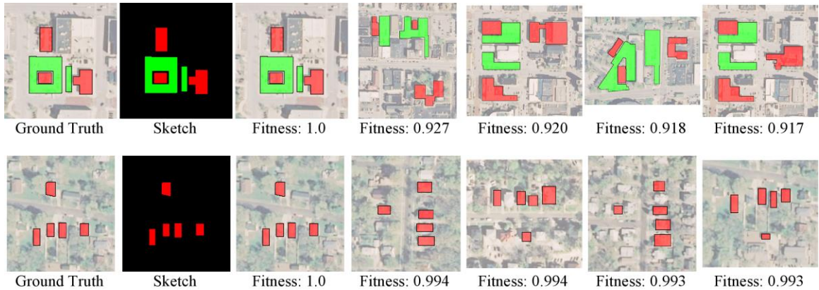
Figure 4.5 Examples of top matches for the resubstitution sketches. Buildings are shown in red and parking lots are shown in green. In both examples, the top match is the correct mapping to the ground truth set, and the remaining high scoring matches all share similar spatial configurations.
